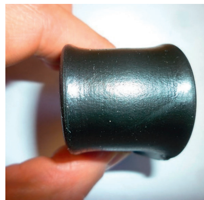
Fig. 4. Rubber-bitumen compound prepared with the planetary roller extruder © Entex
